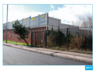
**13. Springmartin Road (Owner: DoJ. Built: 1990 & 1994):** Two pairs of 3.5 metres high security gates approximately 50 metres apart, and with palisade fencing on either side, can be used to close access between Springmartin Road and Springfield Road.
